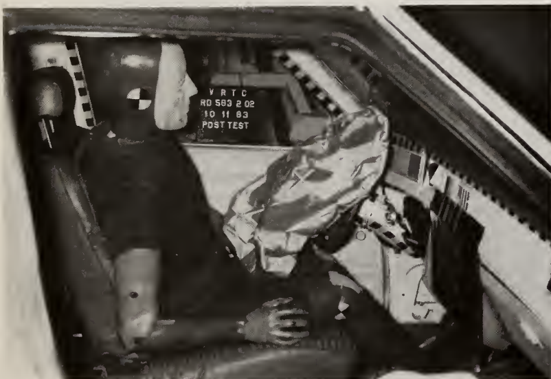
Dummy Position and Steering Wheel Deflection Test 2
